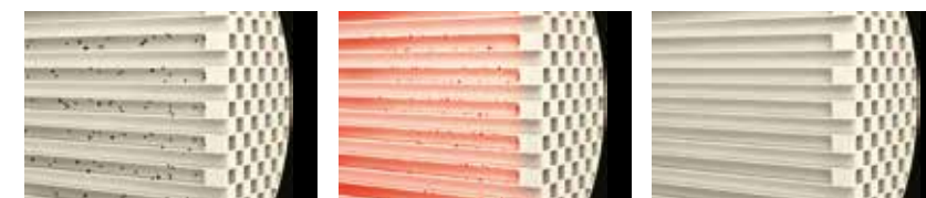
1. Particulate matter trapped 2. Regeneration starts 3. Regeneration completes*
